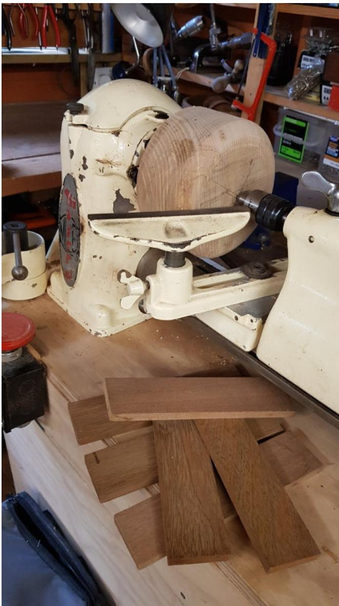
The connection with Frank Procter is now revealed. 6 or 7 flooring tiles working as far as was possible, light, dark, light etc., were glued and clamped then, when set, turned to shape. The third was turned off centre to obtain a different effect.
